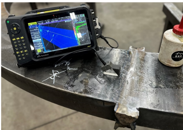
Figure 2 – VEO3 in use on a double V shop butt weld
