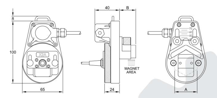
CREO Slim Scan has been developed to allow full encoded scan of studs and bolts where there is limited access. Slim Scan can be quickly attached by the magnetic stop locating on the flats of the nut. The magnetic stop is adjustable to accommodate all nut sizes between 36mm to 65mm A/F. This covers the metric sizes M24 to M42, Imperial sizes 1" to 15/8".
