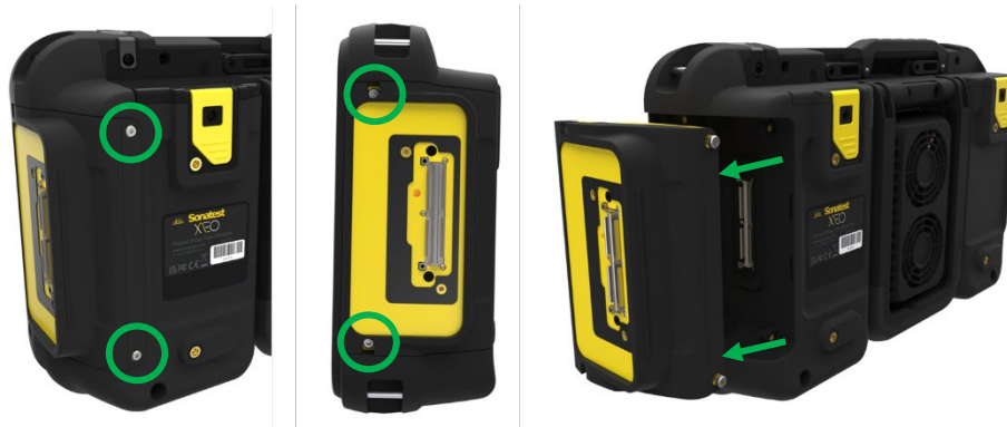
Figure 4 – Changing Mini-docks (Screw Locations)
