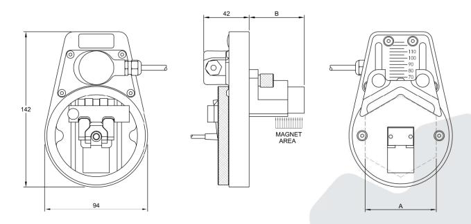
CREO Slim Scan has been developed to allow full encoded scan of studs and bolts where there is limited access. Slim Scan can be quickly attached by the magnetic stop locating on the flats of the nut. The magnetic stop is adjustable to accommodate all nut sizes between 65mm to 128mm A/F. This covers the metric sizes M42 to M90, Imperial sizes 1 5/8" to 3".
