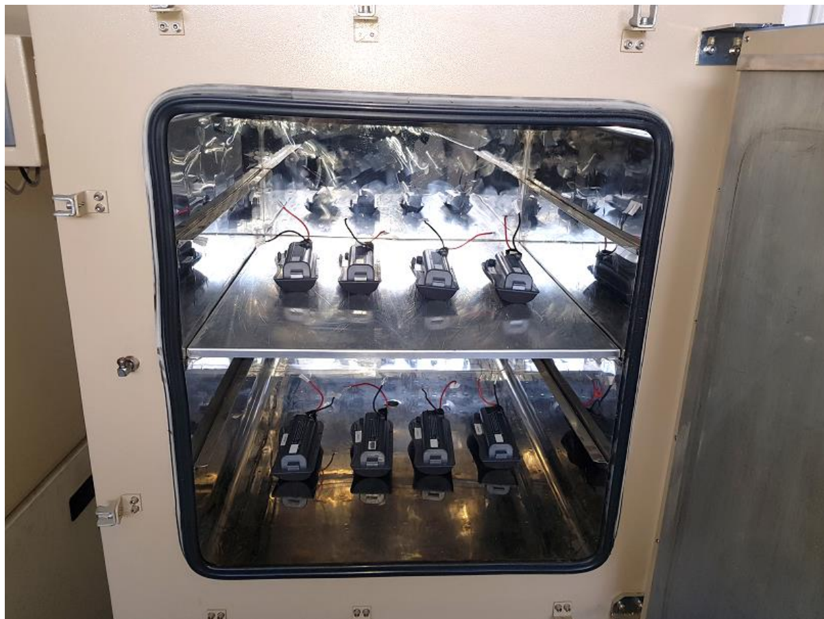
Picture 8: Samples in vacuum chamber
