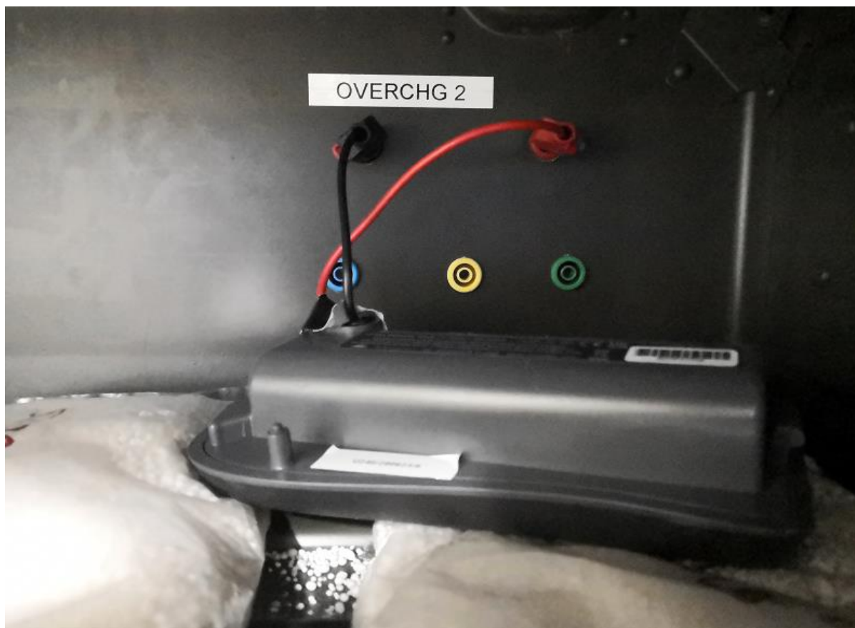
Picture 13: Sample connected to power source
