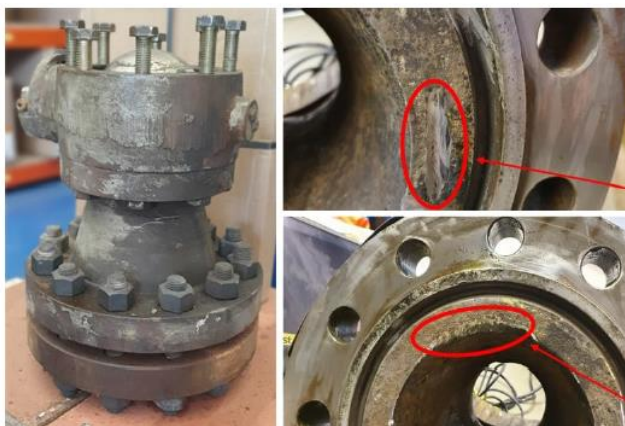
Figure 1 – Flange face defects
