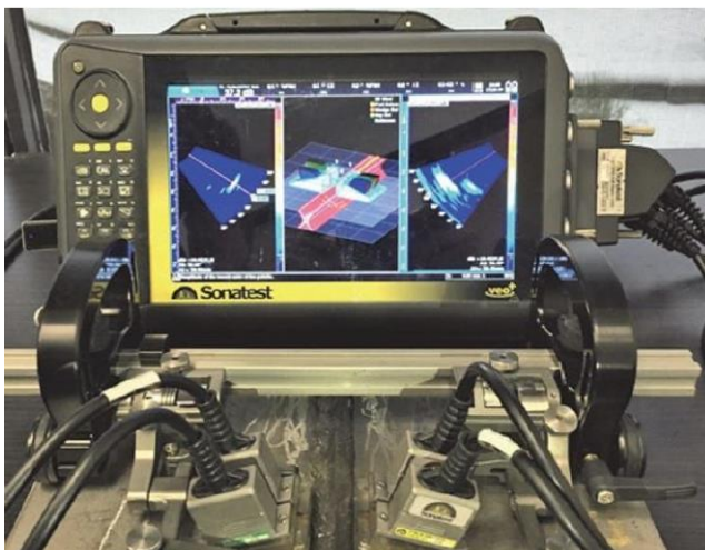
Figure 1 – DLA scanning setup
