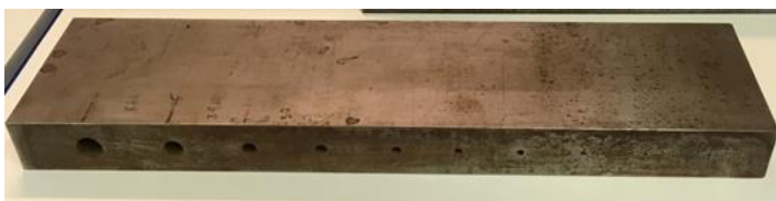
Figure 1 showing the test block and side drilled holes used in the study, the holes can be seen to decrease in size from left to right.
