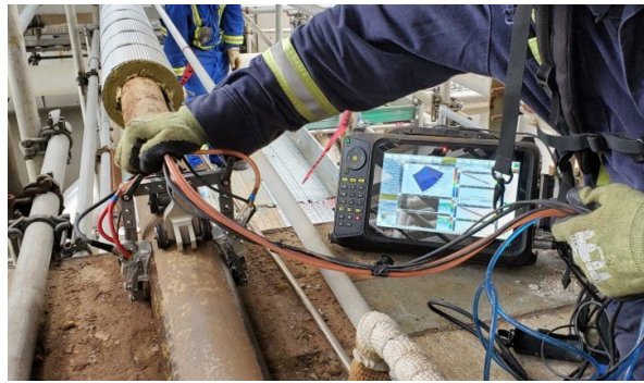
Figure 2 – PA-CAT™ scan being carried out with the VEO3
