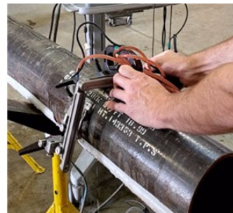
Figure 1 – PA-CAT axial and circumferential scan configurations
