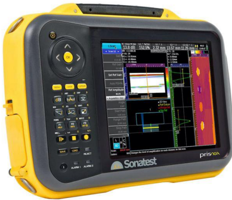
Figure 1 – the PRISMA showing a corrosion mapping layout
