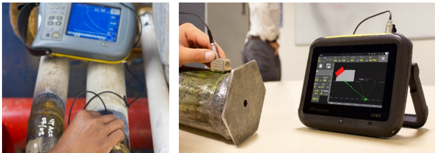
Figure 1 – Ultrasonic butt weld inspection using Sonatest Flaw detectors.
