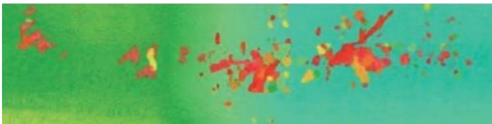
Fig 3 – C-Scan Time-of-flight image
