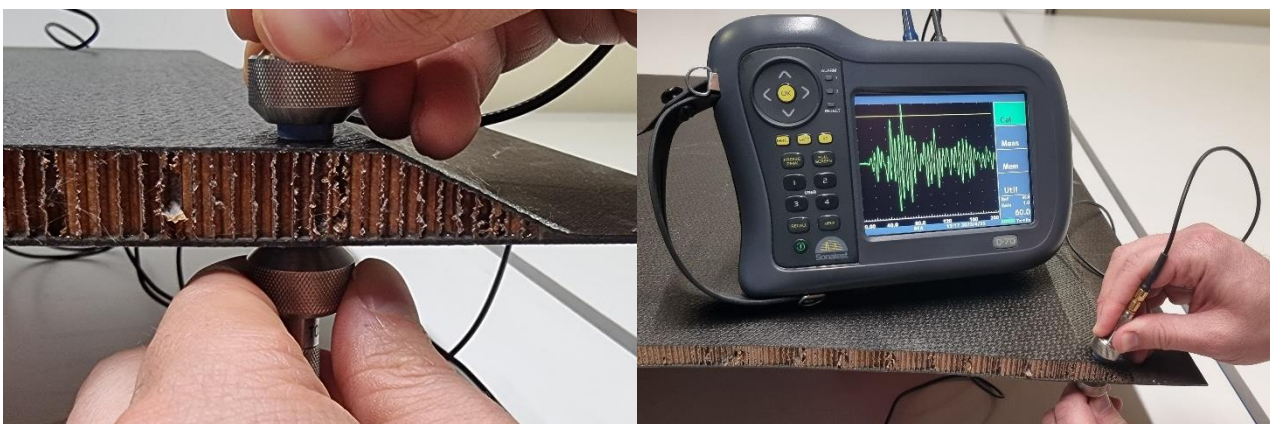
Fig 4 – Through Transmission Technique
