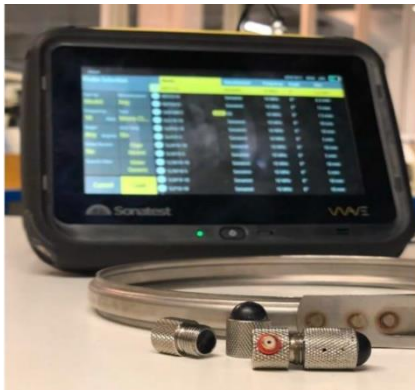
Figure 1 – Spot weld transducers and rubber ball tips
