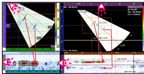
Fig. 1: Typical wrongly produced top view (left). Top view with correct representation (right).
