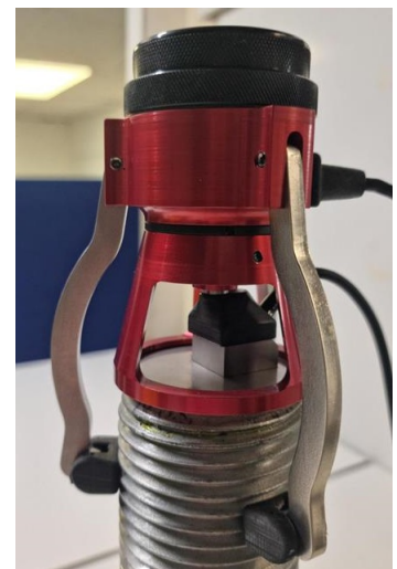
Fig. 3 - Probe and scanner positioned on the bolt
