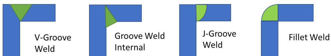
Figure 4 Corner joint: possible weld geometries
