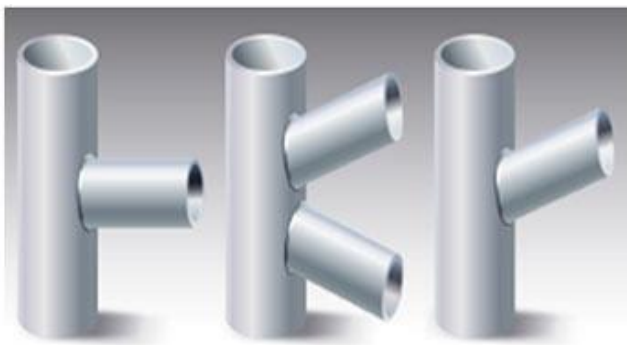
Figure 3 T, K and Y tubular joints.
