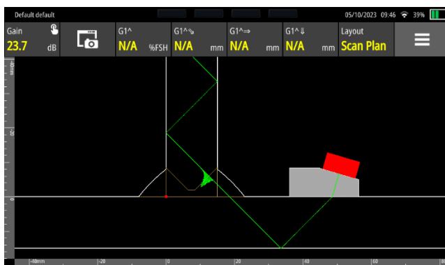
Figure 3 - showing toe crack detection on the WAVE and an example of toe cracking of a T-joint,
