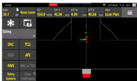
Figure 1 – showing the WAVE scan plan for detection of the unfused land in a T-Joint as highlighted in the right image
