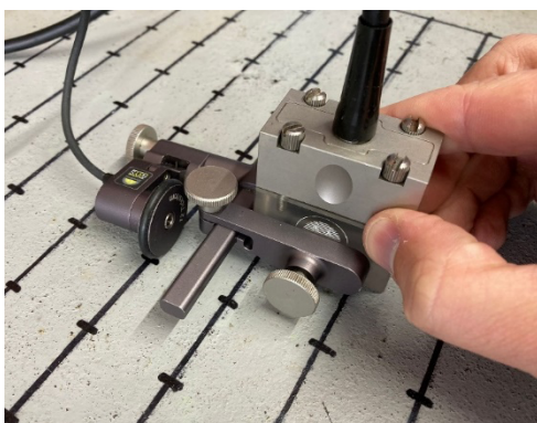
Figure 2 – Encoded manual scan on steel plate
