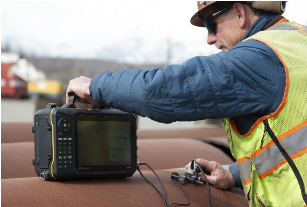
Figure 1 – VEO3 corrosion mapping of steel pipes
