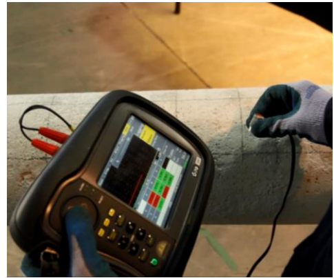
Figure 5 – UT Acquisition Kit
