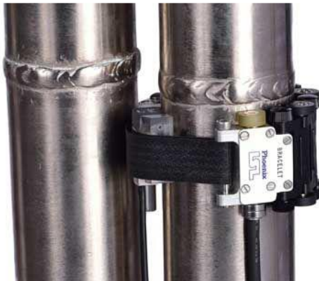
Figure 1 – Bracelet Scanner in a single sided inspection setup
