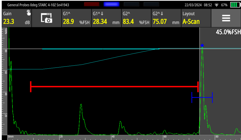
Figure 2 – Video showing Efficient Back-wall Monitoring with BEA ( click here to see a video )
