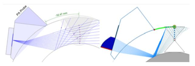
As shown above, one can easily see that the method allows assuring focusing and imaging optimisation for the region of interest defined by the inspector, insuring proper and precise flaw location.
