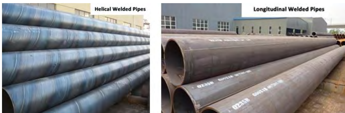
Figure 2 Spiral and longitudinally welded pipes.
