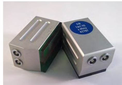
Figure 35: Twin crystal compression angle probe
