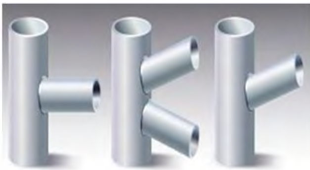
Figure 3 T, K and Y tubular joints.
