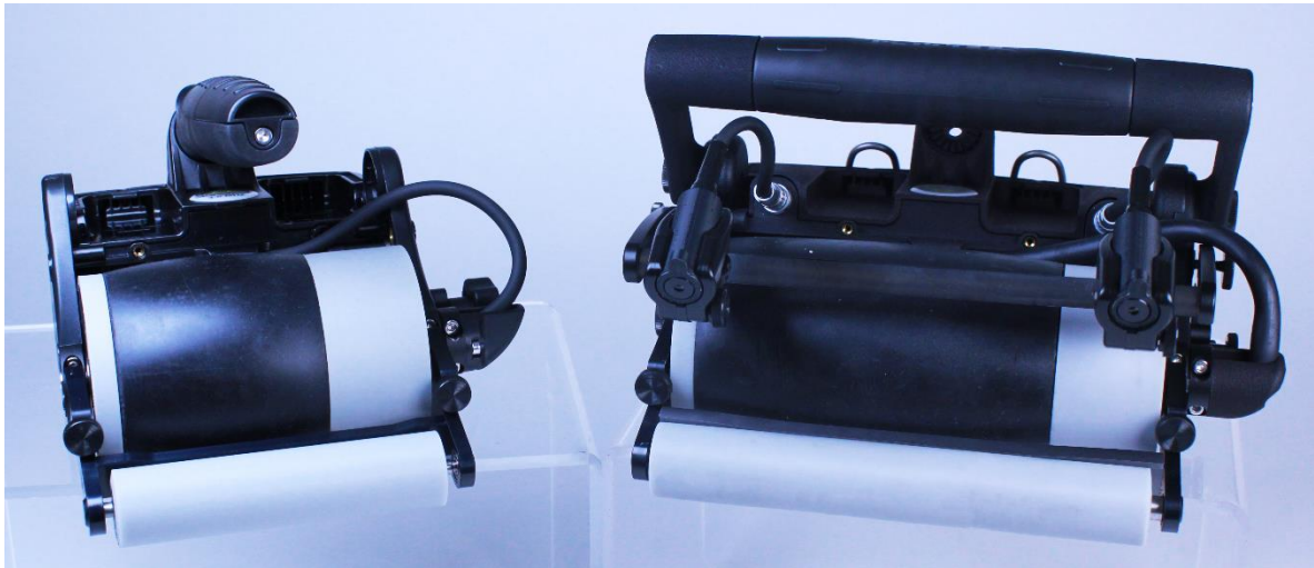
Figure 3 - Wheel Probe 2 is available in 64 element and 128 element versions
