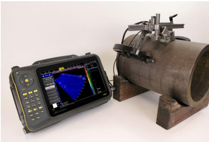
Figure 1 – long seam weld semi automated scan setup
