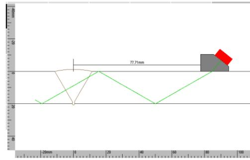
**Figure 28: 'Third-leg' scan - only a bit further up**
