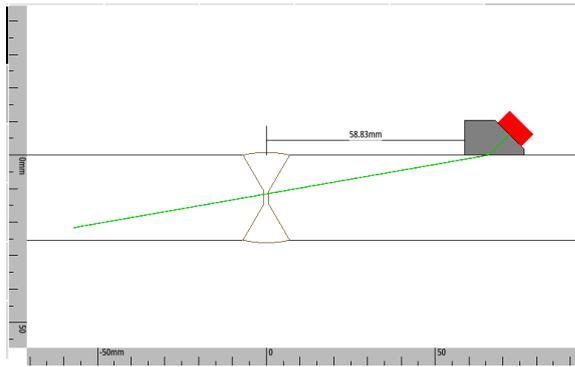
**Figure 33: Single probe inspection for root defects**
