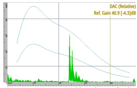
**Figure 19: DAC curve used for echo amplitude evaluation.**
