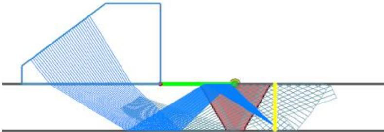
**Figure 40: Phased array sector scan of weld**
