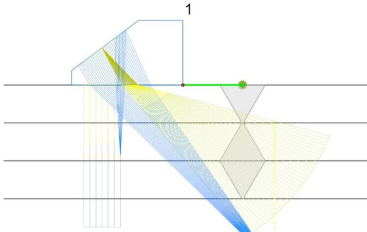
**Figure 46: Use of a coupling check scan**
