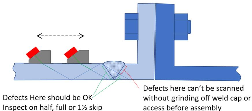
**Figure 17: Example of weld location making inspection difficult**
