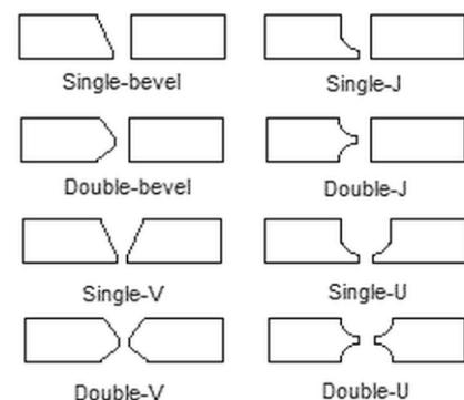
Figure 3: Typical Weld preparations
