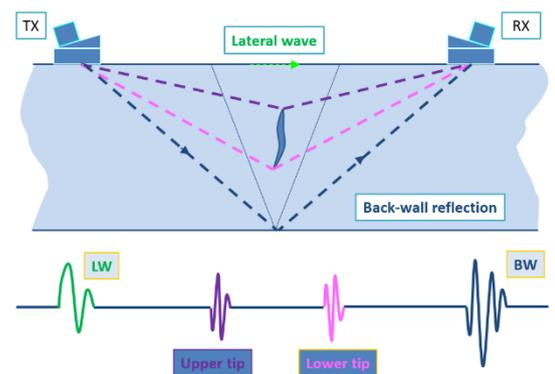
**Figure 36: TOFD measurement**
