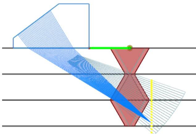
**Figure 41: Phased array sector scan as in the previous figure, shown with reflections in part 'unwrapped'**
