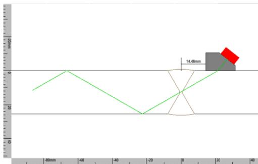
**Figure 31: Nearest scan extent for double-V weld**
