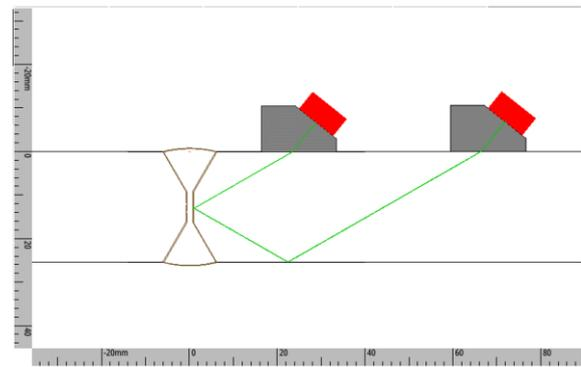
**Figure 34: Tandem probe inspection for root defects**
