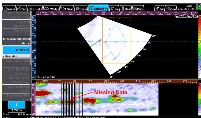
**Figure 47: Missing data due to fast or erratic probe movement**
