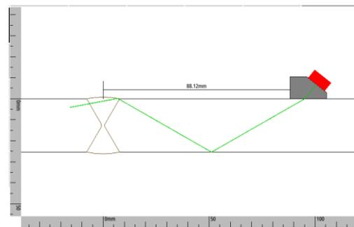
**Figure 32: Furthest scan extent for double-V weld**
