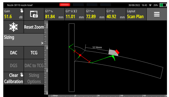
Fig. 4 – Lack of Side Wall Fusion Indication
