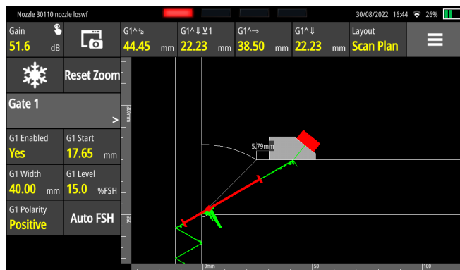
Fig. 3 – Lack of Root Penetration indication
