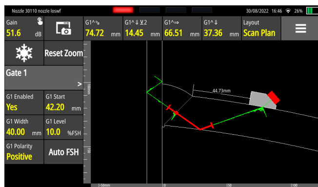
Fig. 5 – Side Wall Crack
