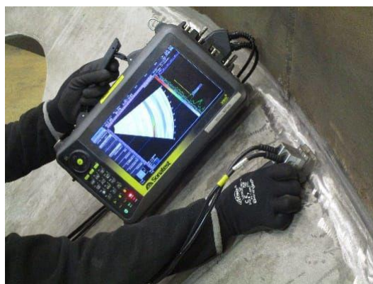
Figure 2 – Manual DLA inspection of welds
