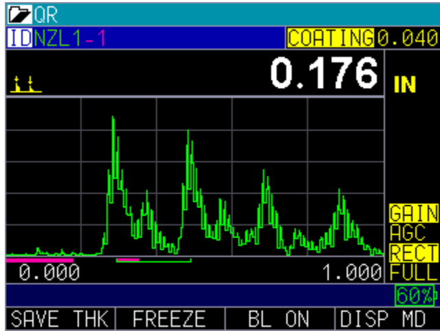
Figure 2 – A-scan display showing the coating thickness in yellow in the top right, and the material thickness in white in the top right
