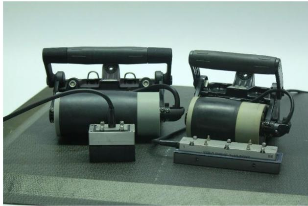
Figure 3: WP2 128 element and 64 element versions shown with Sonatest's other composite inspection probe options, X3 Glider and the X6B Hydroglider
