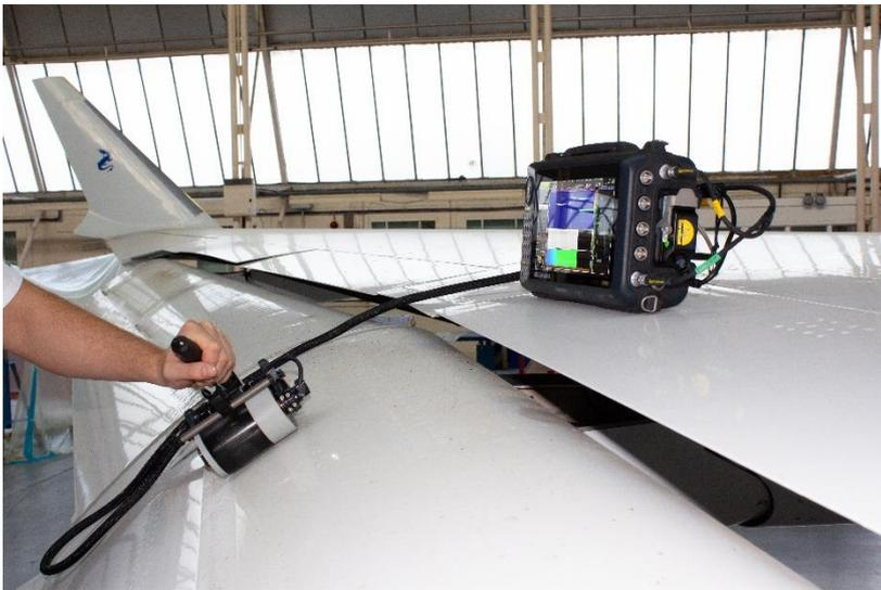
Figure 1: The WheelProbe 2, with its patented rubber design, adapts to all kind of composite materials
