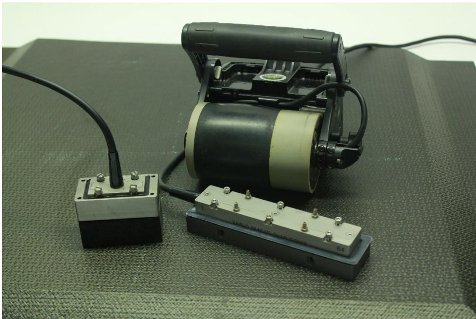
Fig 8 – Phased array probes used for L-Scans, WP2, X3 Glider, X6B with bubble column
