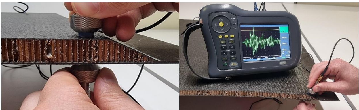
Fig 11 – Dryscan through transmission of composite honeycomb sandwich structure
