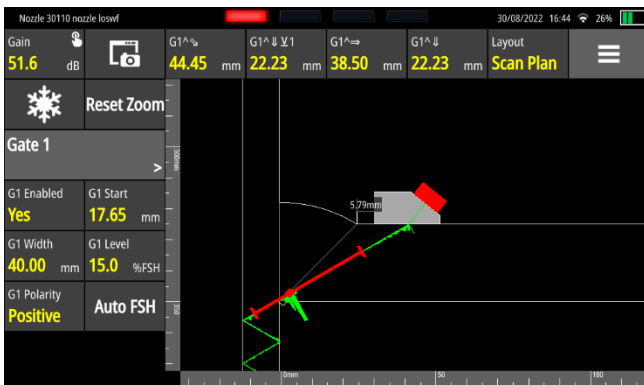
Figure 3 – Lack of Root Penetration indication
