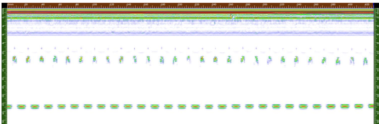
Figure 3 – B-Scan showing the backwall and reinforcement cords
