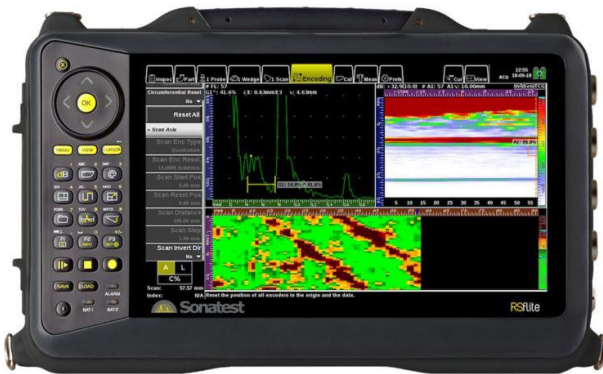
Figure 1 – The RSflite workflow is optimised for composite inspection
